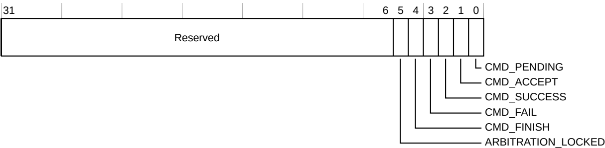
Figure 4-12: STATUS register bit assignments
